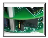
The factory jumpers are shipped connecting the 2 **NO** pins together. Contacts will be open when there is no gas alarm, and will close when a low or high gas alarm is detected.
