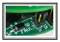
The factory jumper is shipped connecting the 2 **OF (Open on Fault)** pins together. The fault contact will be closed when there is no fault detected in the gas detector. The fault contact will open when any internal fault condition occurs in the gas detector. The fault contact will also open if the 24 volt DC power supply to the detector is interrupted.
