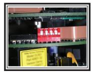
The User Option Switch number 4 sets the operation of the LOW and HIGH alarm LED's and relays.
