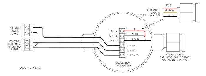
This setup uses three wires between the sensor and the associated control modules. These wires carry the 24 VDC operating power for the sensor, and transmit the 20 mA signal to the controls.
