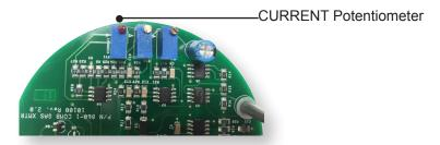
The CURRENT Potentionmeter provides the 170 mA heater current required by the sensor. This pot is adjusted at the factory based on the sensor requirement. The "pot" is then sealed to prevent any changes to the heater current. No adjustments are required on this pot.
