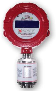
The SST Model GT814 Toxic Gas Detector is a highly versatile and reliable industrial toxic gas detector designed for the toughest job for use in the harshest environments. This detector uses an electrochemical fuel cell sensing element, and provides accurate measurements in all atmospheres. A high reserve of electrochemical activity insures a long life and excellent temperature stability. The performance is relatively unaffected by humidity, providing that conditions are non-condensing.
