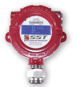
The SST Model GC804 Combustible Gas Detector is a highly versatile and reliable industrial gas detector designed for the toughest job and able to be used in the harshest environments. This detector uses a catalytic poison resistant sensing element which provides accurate measurements in atmospheres where traces of silicone or other poisoning agents may be present and provides excellent long-term zero and sensitivity stability. Readings are unaffected by humidity or carbon dioxide.
