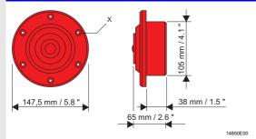
X = 6 x holes dia 5.3 (0.2") and c'bored 10.2 (0.4") equispaced on a 124 mm (4.9") PCD
