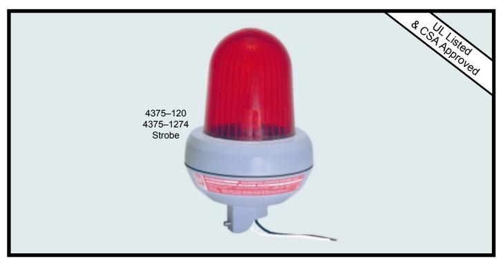
The model 4375 strobe light is UL listed for use in Class I, II & III, Division 2 hazardous locations. Division 2 locations are defined by the NFPA as shown below. These units have a tempered glass lens and are suitable for use in outdoor locations. They may be operated in any position and feature a 3/4" IPS pendant mount.
