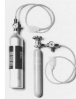
The refillable cylinder type calibrator is for use only with combustible gas sensors. Each refillable cylinder contains 3.6 cubic feet (103 liters) of test gas, which provides approximately 120 normal calibrations
